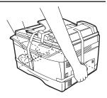
Remove all pieces of tape shown in the illustration below and then open the RSPF and remove the protective materials. Take out the bag containing the TD cartridge.
